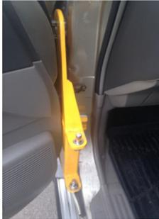
Speedy bar is the part that will hold the main lifter. Insert on to door hinge and make sure it sits properly. Speedy bar should be removed from the door hinge before you shut the door.
