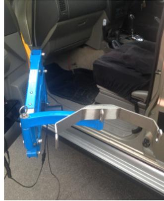
3. Connect main body lifter to the battery
