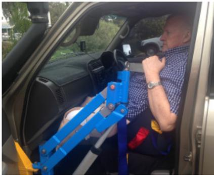
10. Remove lifter, battery and speedy bar. Leave sling under the passenger ready for unloading
