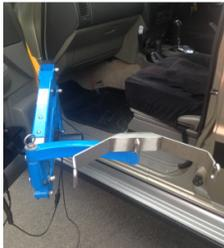
Main body lifter is the part with the engine contains extension arm and lift arm.
