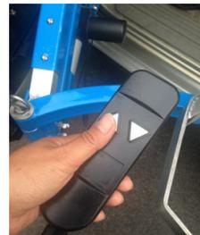
Button up and down. Releasing button will stop from lowering or lifting
