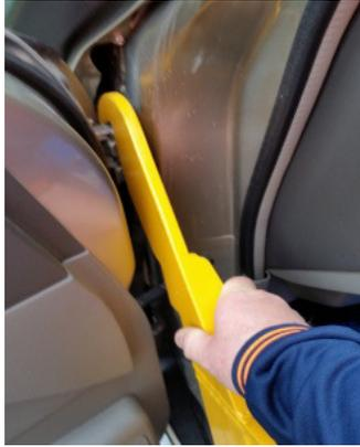
2. Attach main body lifter onto speedy bar
